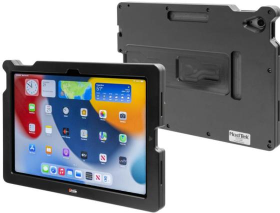
The ModTek Hard Case allows for a direct USB-C connection between the tablet and the dock. USB-C has become the industry standard for mobile devices. Unlike pogo pins, which are susceptible to dust, dirt, moisture, and bending, USB-C offers superior protection and enhanced data capabilities. ModTek enables connections up to 5Gbps with backward compatibility to USB 2.0 devices, while simultaneously charging the tablet.
